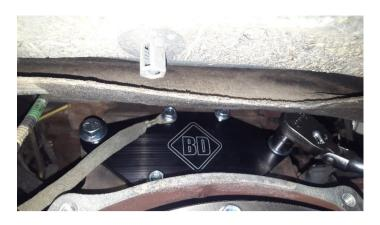
If your truck has a TCC crossover tube, DO NOT try to slip the plate between the tube and the block, this may cut the O-ring.
