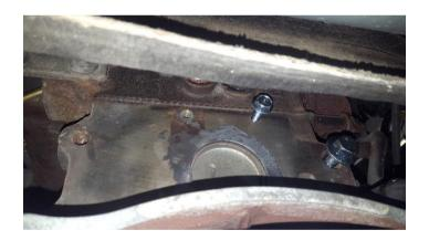
Use some silicone grease and lubricate the O-ring before inserting it into the plate. This ensures the O-ring seats properly on the face.
