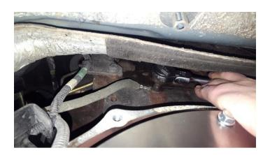
Use an abrasive pad to remove all rust and debris. The plate must sit flush to the motor.
