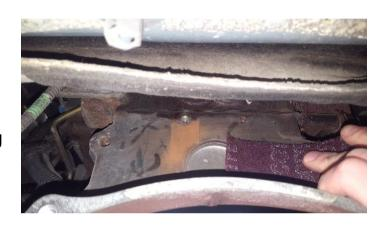
Make sure the M8 and M12 bolts can be threaded in by hand. You may need to run a thread chaser down the bolt holes or use penetrating fluid.
